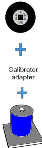
*Figure 32: mounting HealthVib sensor unit on calibrator/shaker*
