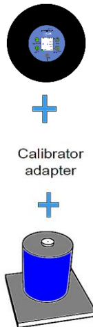
Figure 30: mounting HealthVib sensor unit on calibrator/shaker
