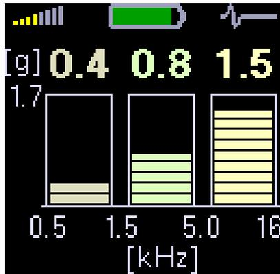
When we need to find the failure on not simple machines (e.g. gearbox) then it is very useful to know the vibration values in several frequency bands.
