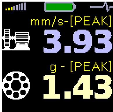
Similar rules for evaluation of the measured values, as in the previous screen are valid for this screen with one difference. The peak (PEAK) vibration values are displayed. It is highest measured value in certain time, which is important for transient shock events evaluation, especially in cases of incipient bearing defects, like:
