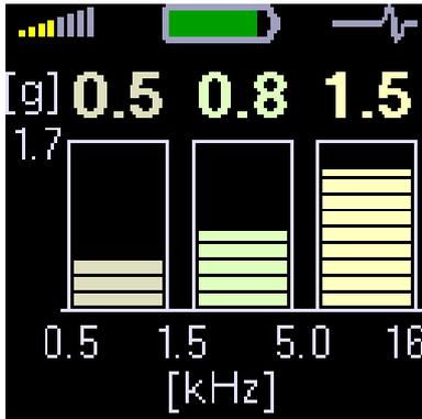
**Vibrations in frequency ranges – gearbox/bearing**
