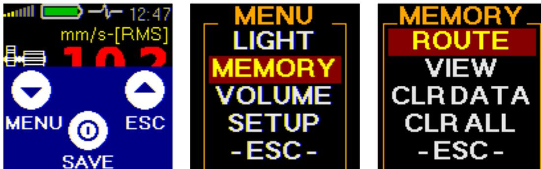
The first machine appears. The machines are the first level of route. By using the < -, + > you can find required machine. When you open one machine (**SEL**) then first point appears (the point level). After you select one point (**SEL**) then all required measurements will be taken.
