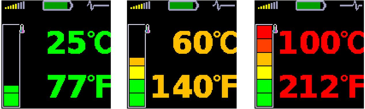
**Temperature measurement** is displayed in Celsius and Fahrenheit degrees. Also the coloured bar is used. The bearing symbol on the other displays is also coloured according to the actual temperature value. The ranges of colours are for less than 30°C - green, 30-45°C - yellow, 45-60°C - orange, 60-75°C - red and for greater than 75°C – dark red.
