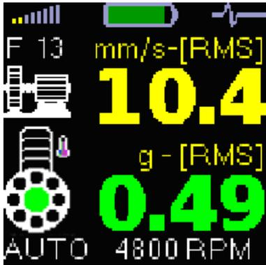
Chosen standard is displayed above the machine symbol (F13 in this case). If Adash standard is chosen, nothing is displayed.
