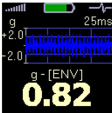
The time signal of bearing vibrations is displayed.  $g_{ENV}$  value is under the time signal (envelope modulated signal - see Methods for ball bearing condition diagnostics chapter. Caution – the time signal is displayed as a direct record, not after envelope modulation. Look at three basic screens for easy work with this function.
