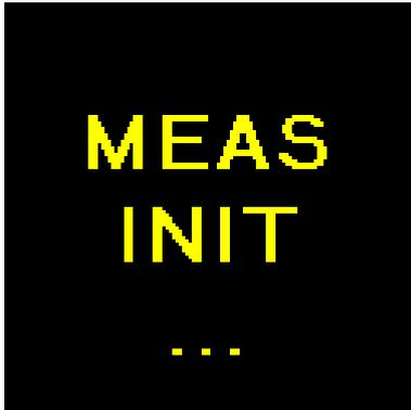
If there is a break in communication between measuring and display boards inside of the instrument, this measurement initialization error is displayed (MEAS INIT). If you see this error, it means that the instrument is malfunctioning and we recommend sending it to the manufacturer for repair.
