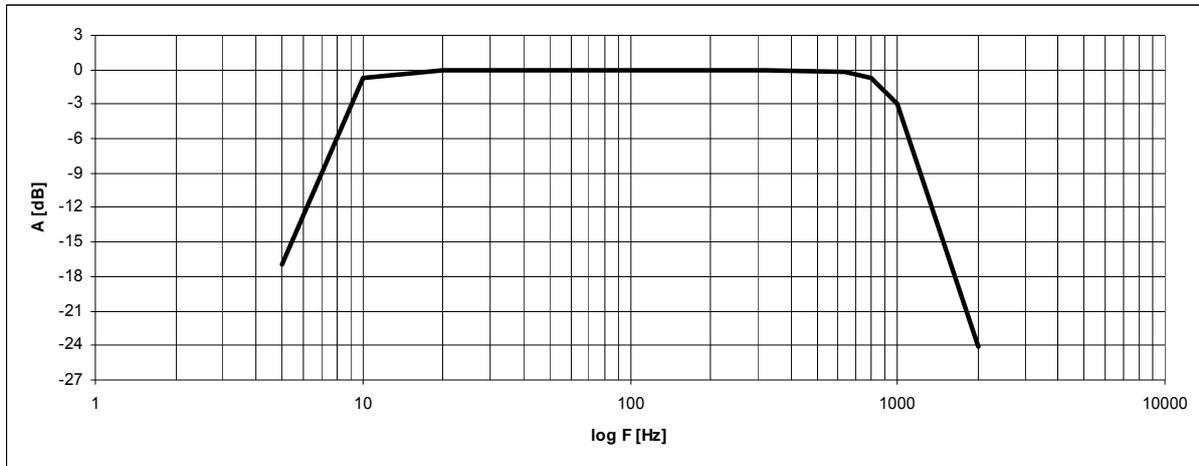
Measurement accuracy (10 mm/s RMS input signal) is +/- 2,5 % (5-500 Hz frequency range) and +/- 5% (500 – 2000 Hz range).
