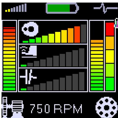
In the left bottom corner you see the Machine icon. The vertical bar displays the general (overall) machine condition. This condition can be evoked by many reasons. The unit evaluates the severity of 3 sources, which are the most occurred in the practice:
