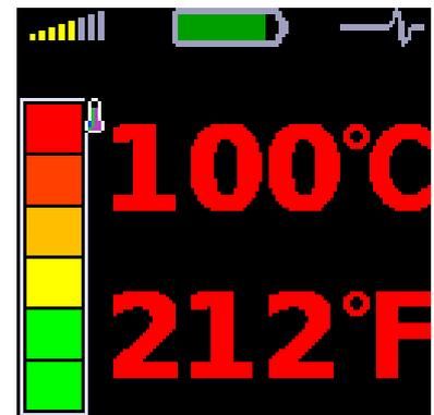
Measured temperature is displayed in Celsius and Fahrenheit degrees. Also the coloured bar is used. The bearing symbol on the other displays is also coloured according to the actual temperature value. The ranges of colours are for less than 30°C - green, 30-45°C - yellow, 45-60°C - orange, 60-75°C - red and for greater than 75°C – dark red.
