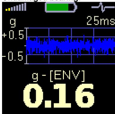
This bearing generates a low amplitude noise only, whose time record shape is steady. It's necessary to have a look on the range of the graph (left side). Signal could look high but it's not when the graph range is low (for instance 0,5 g).
