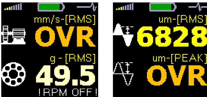
When the value exceeds the range of display, then OVR is displayed.
