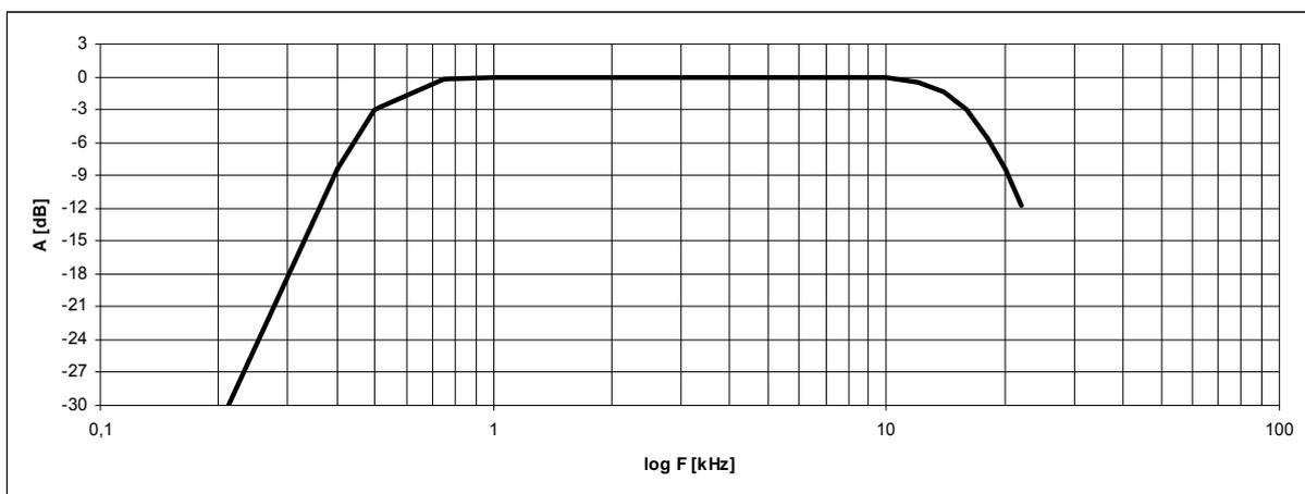
Measurement accuracy (1 g RMS input signal) is +/- 2,5 % in 0,2 -20 kHz frequency range.
