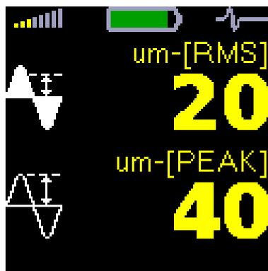
**Overall RMS and Peak displacement** values in the range 2-100 Hz in mm.
