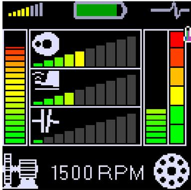
In the left bottom corner you see the Machine icon. The vertical bar displays the overall machine condition. This condition can be evoked by many reasons. The unit evaluates severity of 3 sources, which are the most occurred in the practice:
