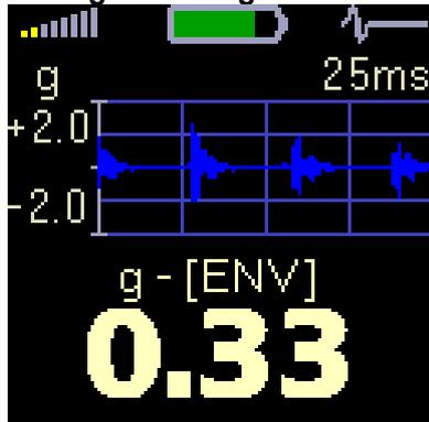
There are clearly visible shocks caused by a rolling element coming across the damage like pitting or crack here. The shocks repeat themselves regularly. The range of the graph is different again (2,0 g in this case).
