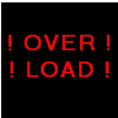
If an input signal is too strong (higher than 12V peak), the instrument cannot process it, the overload error is displayed. The instrument is not capable of measuring this signal.
