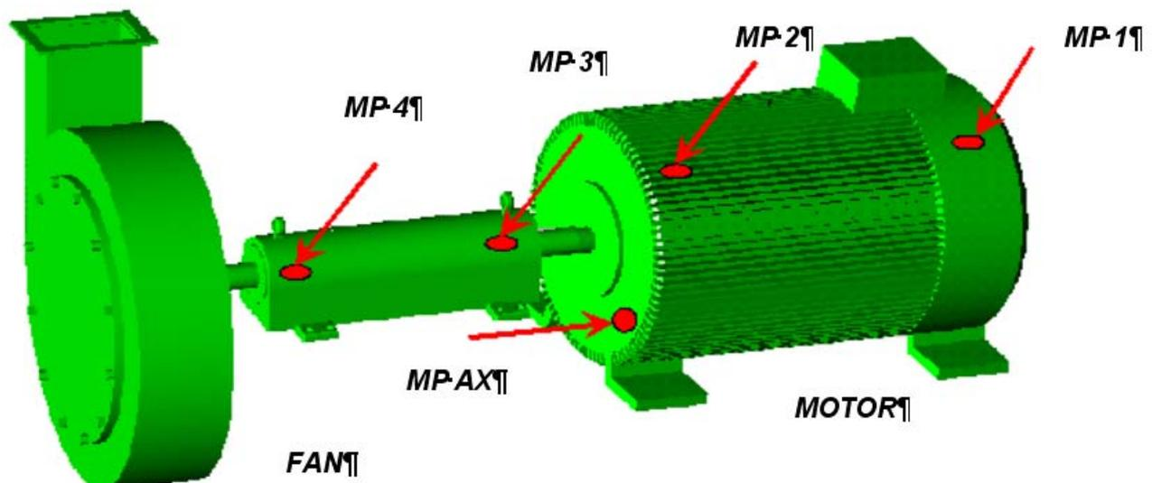
For the measurement in radial direction, we are going to place the sensor perpendicularly to the axis of rotation, for axial measurement along the axis. The radial measurement can be usually performed horizontally, vertically or in another angle. The importance of the angle choice should not be overstressed; choose any radial direction with easy access.
