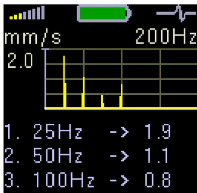
This screen is important for detection of the mechanical looseness. When the graph shows a number of lines (typically 3 or 4) with the same space between them and the first line is on the speed frequency (see the value description on the bottom) probably mechanical looseness is the machine problem.
