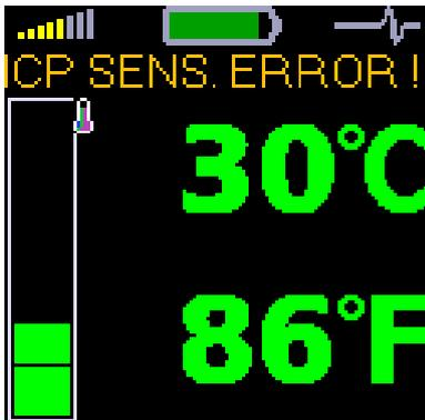
When incorrect connection of a sensor, unsuitable sensor type, broken cable etc. is detected, then the temperature screen occurs and the error message is written upon the values.
