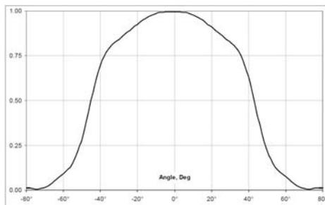
Sensor sensitivity vs. the angle
