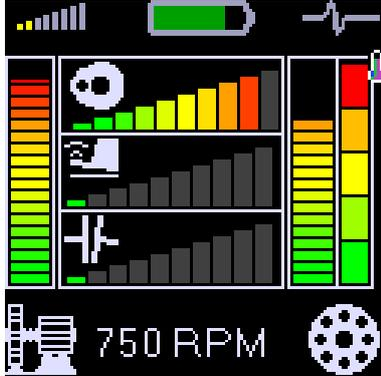
The next three bars are located in the middle. They display the severity level of UNBALANCE, LOOSENES and MISALIGNMENT (from the top).
