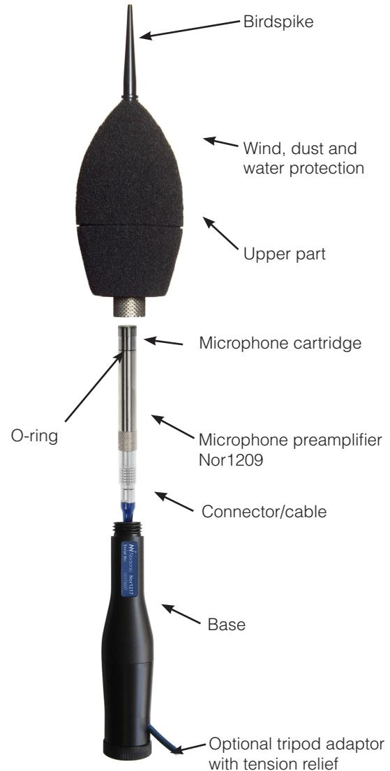
Unscrew and remove the upper part consisting of birdspike and windscreen as one unit. Do not remove the windscreen from this upper part as this may destroy the weather protection and alter the acoustic performance.
