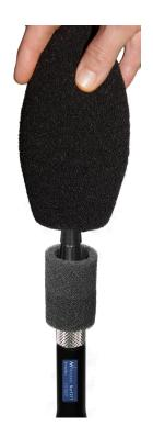
The lower part of the windscreen, the dust mesh and rain hood are not parts that can be serviced by the user. In case of wear or strong contamination we recommend to order a replacement unit (Spare part Nor4560) or send the part to the factory for refurbishment.
