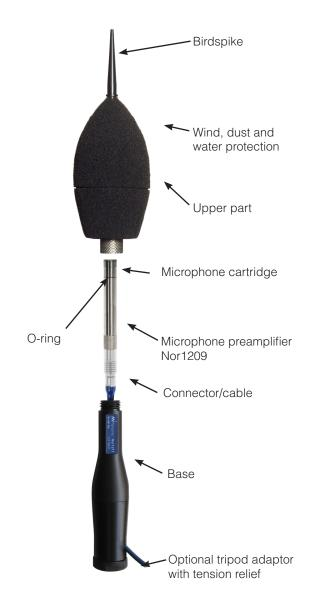
Unscrew and remove the upper part consisting of birdspike and windscreen as one unit. Do not remove the windscreen from this upper part as this may destroy the weather protection and alter the acoustic performance.
