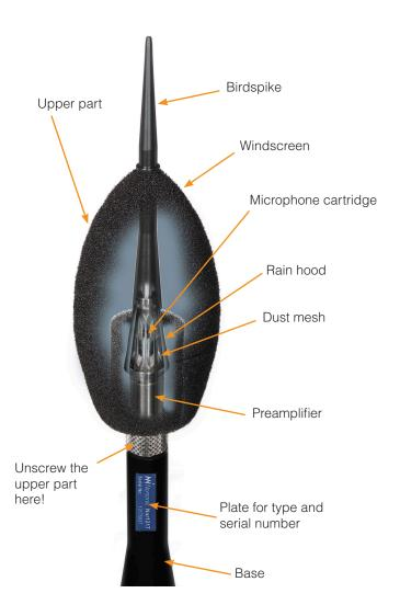
The lower part consists of the base, the microphone cartridge and the preamplifier Nor1209. A normal microphone cable supplied with Norsonic sound level meters, like Nor1408A, should be used for connection to the sound level meter instrument. An adaptor for mounting the outdoor microphone on a tripod is included.
